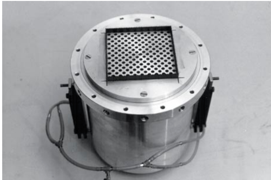
Fig.3. Diaphragm holder with integrated turbulence grid.
